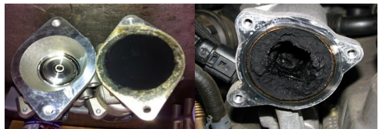
New, partially blocked and heavily blocked EGR valves
